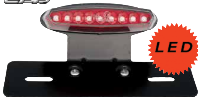
124-TL3 TAIL LIGHT WITH NUMBER PLATE BRACKET RED 9 LED LENS WITH 4 LED CLEAR NUMBER PLATE LIGHTS EMK BLACK
